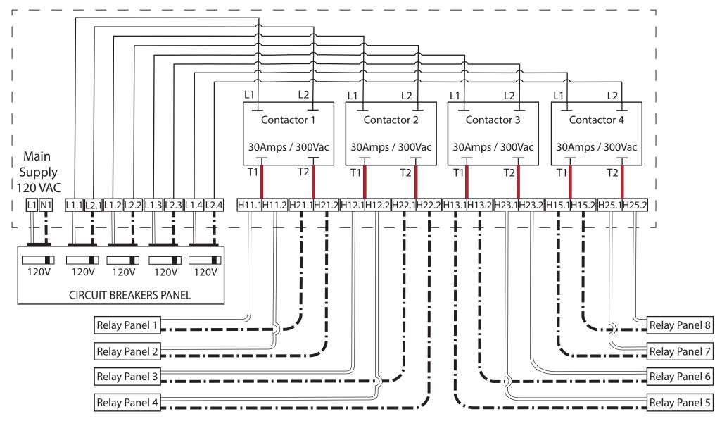
Power Modulator 3 has 4 contactors, each one can take up to 300 VAC, 30 Amp. SCPM can operate up to 4 zones with selectable sequencing method. SCPM has double wire terminals for the load connections. The built-in ground fault protection must be disabled, by disconnecting the two wires connected to the green terminals on the Ground Fault Sensor.
