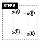
**STEP 6:** Mark A, B, C, and D according to the data from Step 5; It is suggested that this product be installed at least 23.5 inches (59.69 cm) above floor level. (WARNING: The electrical connection should avoid all water). This mounting location must comply with all local building and electrical codes.
