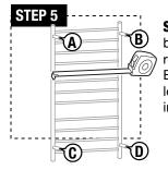
**STEP 5:** Use a tape measure to measure the distance between the center points of each wall bracket tube; record the distances between points AB, AC, CD, and BD. Mounting point C will determine electrical box location. See Electrical Assembly in following instructions.
