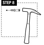
**STEP 8:** Use a hammer to knock plastic drywall anchor (f) into wall completely.
