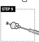
**STEP 9:** Insert long screw (i) through mounting bracket (g), then screw into plastic drywall anchor (f).
