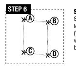
**STEP 6:** Mark A, B, C, and D according to the data from Step 5; It is suggested that this product be installed at least 23.5 inches (59.69 cm) above floor level. (WARNING: The electrical connection should avoid all water). This mounting location must comply with all local building and electrical codes.
