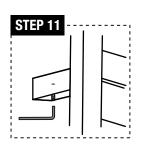
**STEP 11:** As shown in the picture, install the set screws (b) into the hole of all the tubes (a and g) using the allen wrench; fix the tube (a and g) onto the mounting bracket (e).
