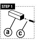
**STEP 1:** As shown in the picture, insert the short mounting screw (c) through the tube in the center of the mounting tube (a).
