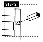
**STEP 2:** Use the short mounting screw (c) to fix the mounting tube (a) to the threaded metal pad on the vertical bar on the back of the towel warmer.
