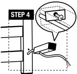
**STEP 4:** Guide the electrical cord through the electrical connection mounting tube (g) and use the long mounting screw (h) to tighten the electrical connection mounting tube to the vertical bar.
