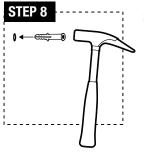
**STEP 8:** Use a hammer to knock plastic drywall anchor (d) into wall completely.
