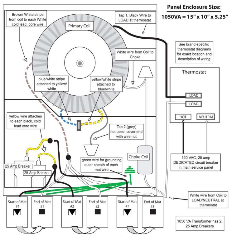
NOTE: The 1050 VA transformer can handle up to a total of 1050 watts of low voltage warming rolls. If the total watts requirements of all the rolls exceeds 1050 watts, a larger capacity transformer will be needed. To avoid nuisance GFCI tripping, please use plenty of electrical tape to prevent arcing between the conductors and their respective braids/ shields.
