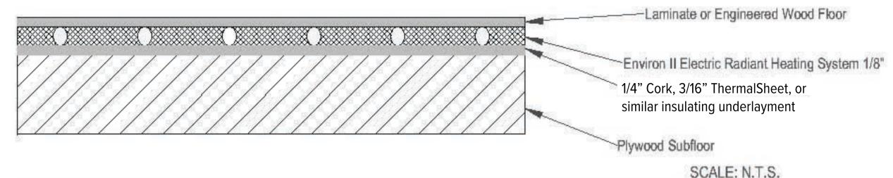
Application: Floating Laminate or Engineered Wood over Wood.
