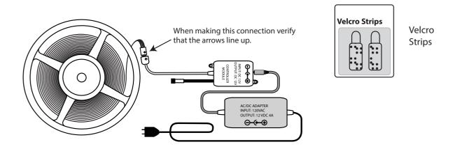
3. Assemble the parts as shown. Test the system to see if it is functioning correctly. Operation instructions come separately. If the unit does not function, please call WarmlyYours Technical Support department at 800-875-5285. If the system operates correctly, disconnect unit from power and disconnect all other connections and proceed to Step 4. Warning: Do not operate spooled LED's for more than a couple of minutes during testing. Spooled LED's can overheat rapidly and damage may result.
