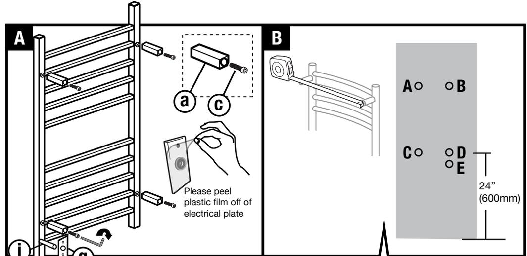
**Note:** Use a tape measure to measure the distance (on center) between the four mounting brackets. Use a pencil to mark locations A, B, C, D and E on the wall according to the measurements. We suggest mounting the Towel Warmer at least 24" (600mm) above the floor. We suggest mounting the left rail of the towel warmer to a stud, if possible.
