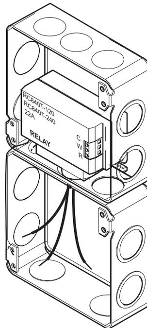
1. INPUT VOLTAGE TO THE RELAY, VOLTAGE OF THE RELAY ITSELF AND THE VOLTAGE OF THE MAT SHOULD BE ALWAYS THE SAME.
