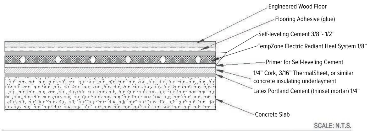
Application: Glued Engineered Wood over Insulated Concrete.
