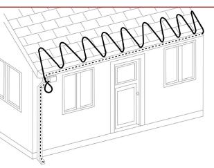
Cut the heating cable to proper length, if necessary. This can be done before or after the cable is on the roof.
