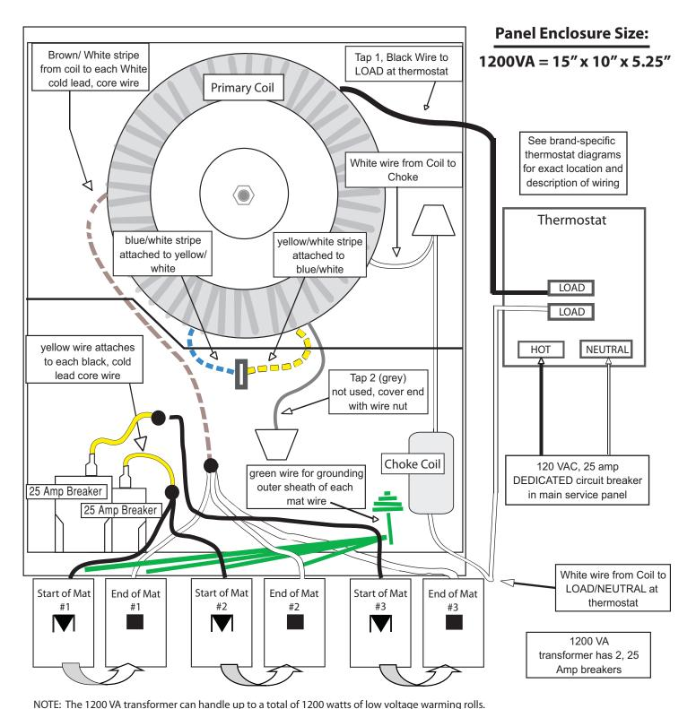
If the total watts requirements of all the rolls exceeds 1200 watts, a larger capacity transformer will be needed.
