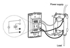
Connect the power base as per the following connection diagram.
