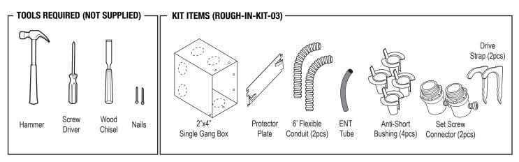
This kit contains enough conduit for protection of the line voltage and low voltage wires. If your local code does NOT require conduit to protect low voltage wires, contact WarmlyYours for kit ROUGH-IN-KIT-02.
