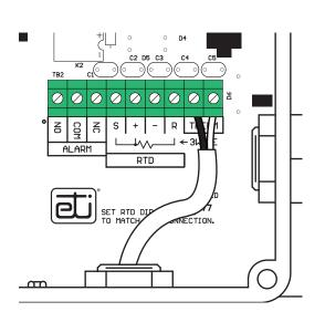
The Thermistor input is not affected by the DIP Switches
