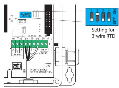
FIGURE 5. Temperature sensor wiring and DIP switch configurations
