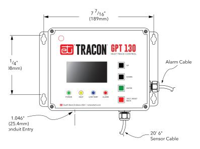
NOTE: Cover screws maximum torque: 4 In-Lbs.
