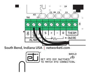
FIGURE 7. External alarm connection
