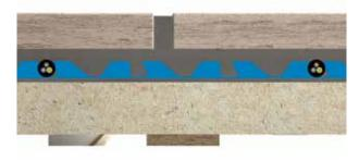
Imitation.Low thermal inertia. Tiles are installed directly on top of the heating
