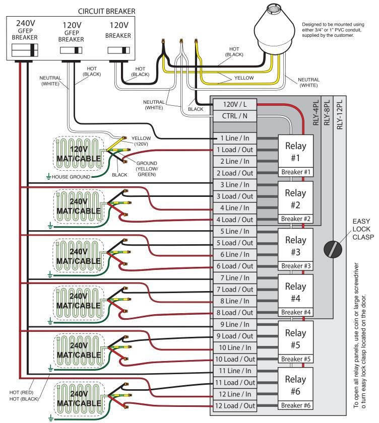
These terminals are suitable for wire gauge 10awg and smaller size wire. Consult local electric code concerning Applicable voltage drop wire sizing. Install in accordance with the requirements of all applicable electrical and Building codes and regulations. Ensure that all conduit/cable terminations are watertight.
