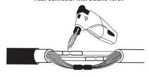
Step 7 - Insert both Ground leads into the uninsulated crimp connector and crimp.
