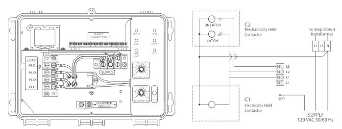
FIGURE 9. APS-3C: Operating Mechanically-Held and Electrically-Held Contactors
