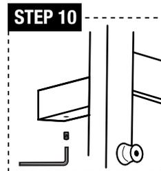
**STEP 10:** As shown in the picture, install the set screws (c) into the hole of all the tubes (a) using the allen wrench; fix the tube (a) onto the mounting bracket (g).
