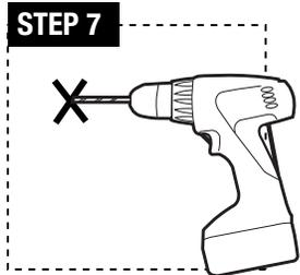
**STEP 7:** Drill A, B, C, and D holes with an appropriately sized bit. Use a hammer to knock plastic drywall anchor (f) into wall completely.
