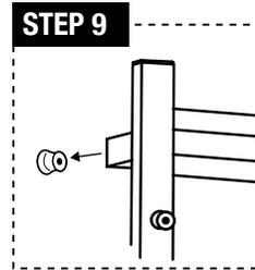
**STEP 9:** Install the tube (a) onto the bracket (g).
