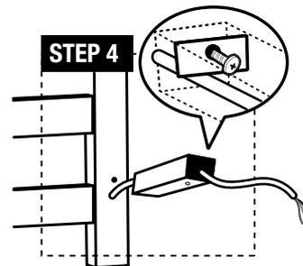
**STEP 4:** Guide the electrical cord through the electrical connection mounting tube (b) and use the long mounting screw (e) to tighten the electrical connection mounting tube to the vertical bar.
