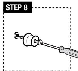
**STEP 8:** Insert long screw (i) through mounting bracket (g), then screw into plastic drywall anchor (f).
