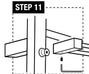
**STEP 11:** Install shelf (k) by inserting the shelf's mounting tube on to the bracket and tighten by inserting the set screw (L) into the hole.
