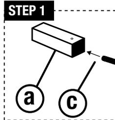
**STEP 1:** As shown in the picture, insert the short mounting screw (d) through the tube in the center of the mounting tube (a).
