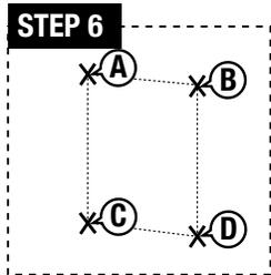
**STEP 6:** Mark A, B, C, and D according to the data from Step 5; It is suggested that this product be installed at least 23.5 inches (59.69 cm) above floor level. (WARNING: The electrical connection should avoid all water). This mounting location must comply with all local building and electrical codes.
