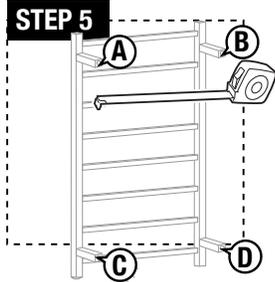
**STEP 5:** Use a tape measure to measure the distance between the center points of each wall bracket tube; record the distances between points AB, AC, CD, and BD. Mounting point C will determine electrical box location. See Electrical Assembly in following instructions.
