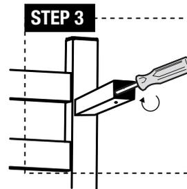
**STEP 3:** Screw down the short mounting screw (d) with a screwdriver. Note that the set screw of the tube (a) should point towards the floor when the towel warmer is wall mounted. Fix the remaining two mounting tubes (a) to the vertical bars with threaded metal pads by repeating Step 1-3.
