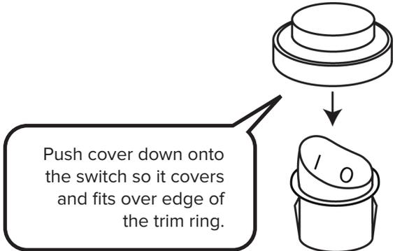
Push cover down onto the switch so it covers and fits over edge of the trim ring.
