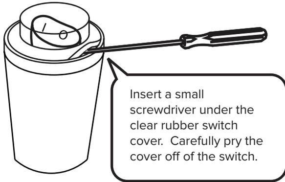
Insert a small screwdriver under the clear rubber switch cover. Carefully pry the cover off of the switch.
