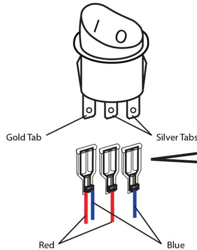
The push-on terminal with the two wires attached to it is attached to the gold tab of the switch. The red push-on terminal gets attached to one silver tab and the blue terminal attaches to the last silver tab. There is no polarity with these 2 connections.
