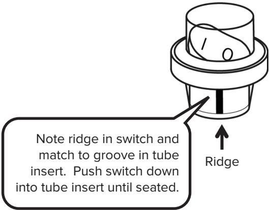
Note ridge in switch and match to groove in tube insert. Push switch down into tube insert until seated.
