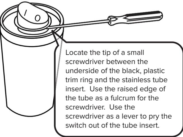
Locate the tip of a small screwdriver between the underside of the black, plastic trim ring and the stainless tube insert. Use the raised edge of the tube as a fulcrum for the screwdriver. Use the screwdriver as a lever to pry the switch out of the tube insert.
