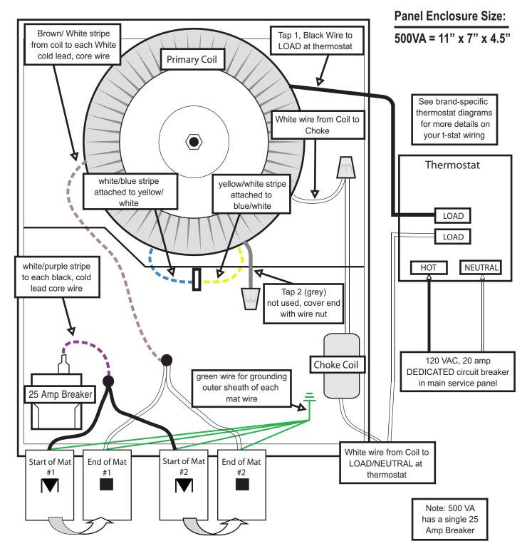
**NOTE:** The 500 VA transformer can handle up to a total of 500 watts of low voltage warming rolls. If the total watts requirements of all the rolls exceeds 500 watts, a larger capacity transformer will be needed. To avoid nuisance GFCI tripping, please use plenty of electrical tape to prevent arcing between the conductors and their respective braids/shields.
