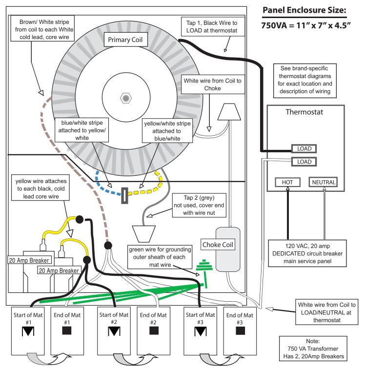
NOTE: The 750 VA transformer can handle up to a total of 750 watts of low voltage warming rolls. If the total watts requirements of all the rolls exceeds 750 watts, a larger capacity transformer will be needed. To avoid nuisance GFCI tripping, please use plenty of electrical tape to prevent arcing between the conductors and their respective braids/ shields.
