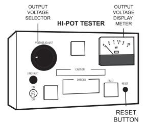
Do not plug Hi-Pot into a GFCI protected circuit. If the Hi-Pot will not reset, and the fault light is illuminated, the circuit that the Hi-Pot is attached to is not wired correctly. Find another available circuit to use. The Hi-Pot will not function without a
