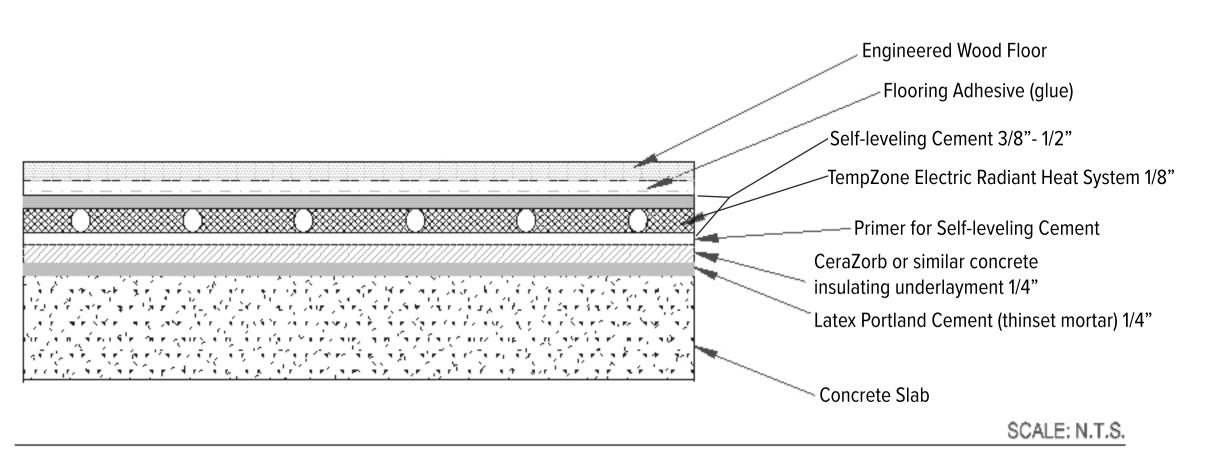
Application: Glued Engineered Wood over Insulated Concrete.
