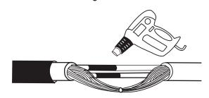
**Step 7 -** Slide the heat shrink tube over the completed joint and shrink it with a hot air pistol. Do not use a naked flame. Verify sealant flow at both ends of the tube. There should be clear glue at each end of the tube. This will ensure a waterproof seal.
