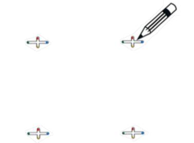
**5.** Drill the holes using a drill bit size that is slightly smaller than the drywall anchor. Then insert the drywall anchors into the holes, and screw the screws into the drywall anchors.
