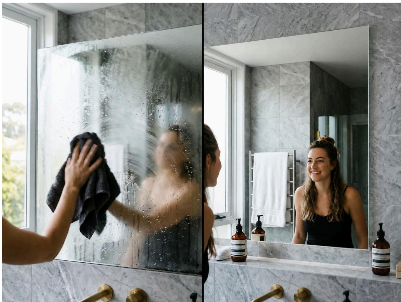
Left: fogged mirror. Right: fog-free mirror with a heated defogger.
