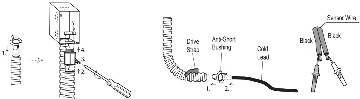
5. Once the electric radiant heating system has been installed, test the system with a digital ohm meter as described in the installation manual. If the system tests good, run the cold lead up the conduit and into the thermostat box.
