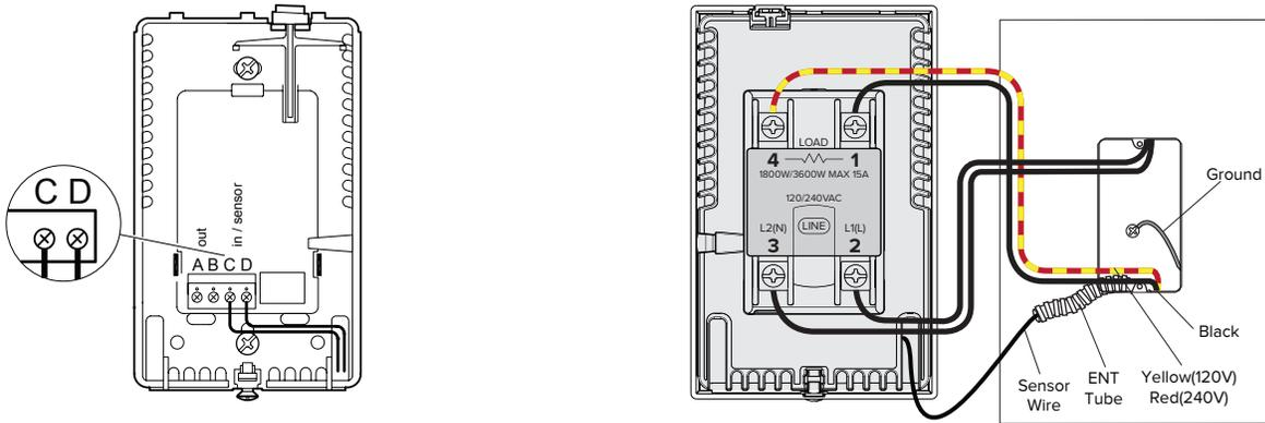
11. Place the thermostat on the front of the white cover plate and line up all of the holes. Use the included screws to attach the power base and white cover plate. Center and level the thermostat and then tighten the screws to hold the pieces in place. Install thermostat's faceplate onto the power base.
