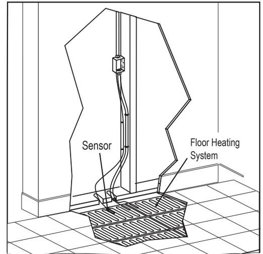
6. Once the wires are run up to the thermostat box, install the cable protector plate so it covers the wires at the bottom plate. This will protect the wires from stray nails.
