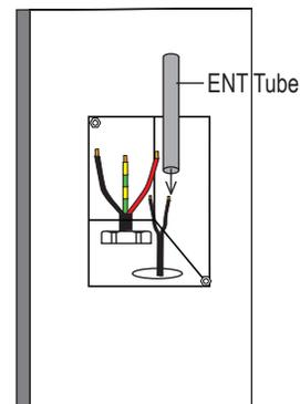
10. Make connections to line and load wires at the back of the thermostat. Place sensor wires into and through the side hole of the thermostat's power base. Attach the sensor wires to the front of the thermostat's power base.
