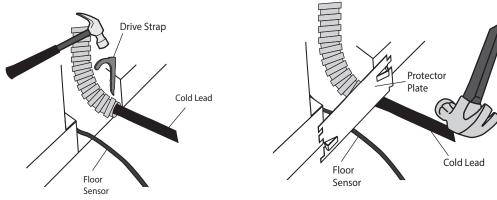
7. Place the smurf/ENT tube over the sensor wire to protect it from the high voltage wires.
