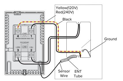
Place the thermostat into the single gang box and line up all of the holes. Use the included screws to attach the power base to the box.
