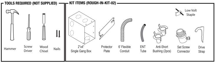
This kit contains enough conduit for protection of line voltage wires.
