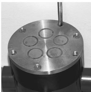
Figure 2. Rotate Height Adjustment Screws
