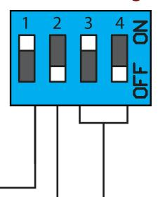
Temperature Sensor Fault Mode
