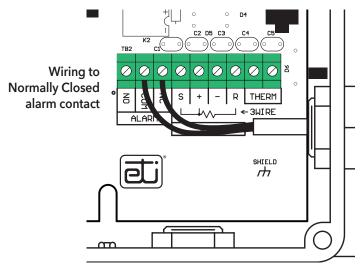
FIGURE 5. External alarm connection
