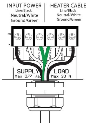
FIGURE 3. Contractor connections.
