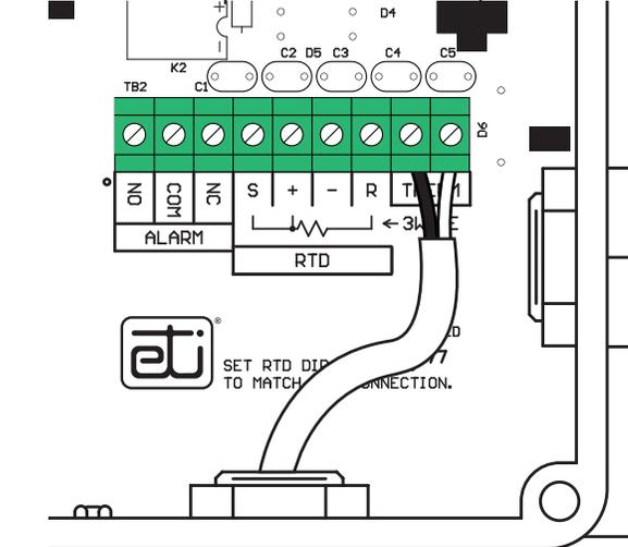
FIGURE 4. Temperature sensor wiring
