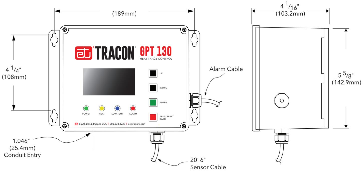
FIGURE 2. Mounting dimensions.
