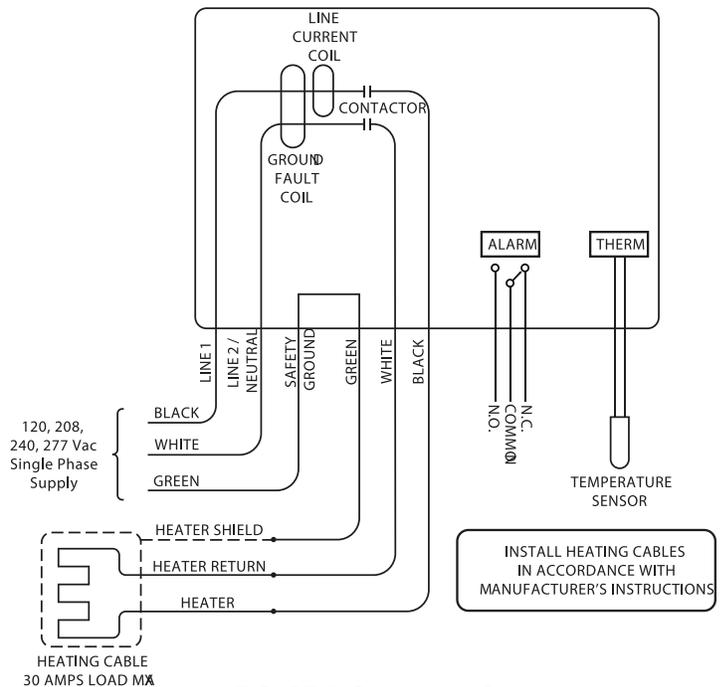
FIGURE 4. Connection Schematic
