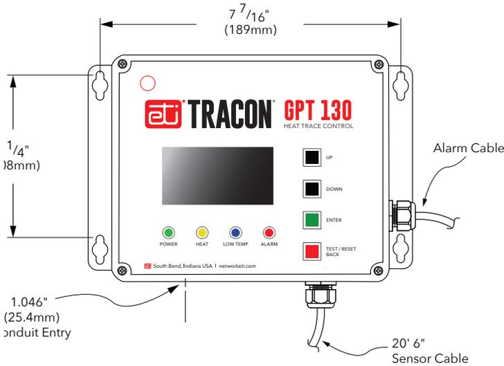
NOTE: Cover screws maximum torque: 4 In-Lbs.
