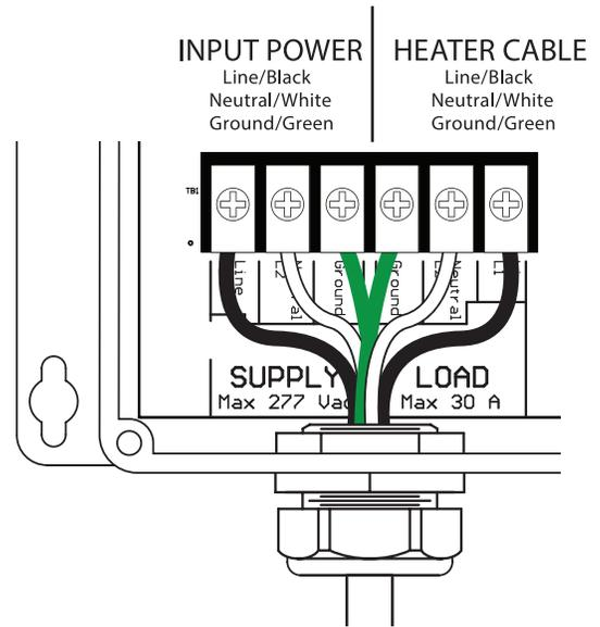
FIGURE 3. Contractor Connections
