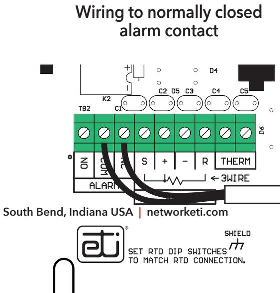
FIGURE 7. External alarm connection
