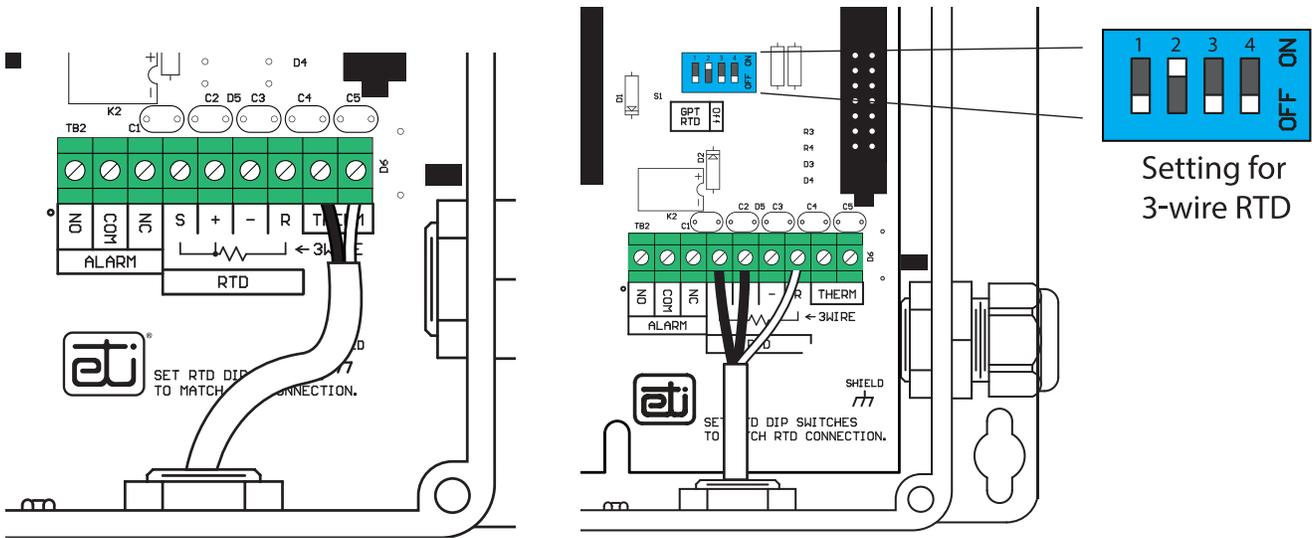
FIGURE 5. Temperature sensor wiring and DIP switch configurations
