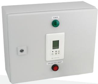
With four contactors, the Power Modulator 3 allows customers to use one per each zone, up to four zones. This can be done in one of two ways. Either all four zones can be used for snow melting, or three zones can be used for snow melting and the fourth zone can be used for roof and gutter deicing.
