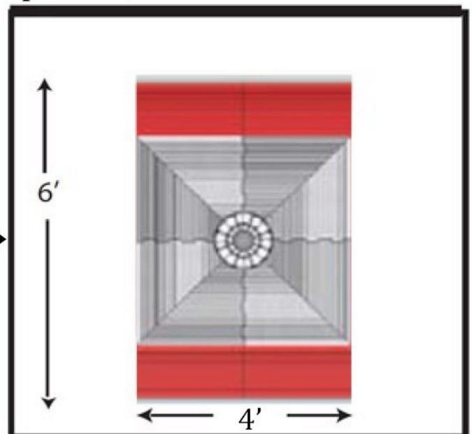
5. The current pan can accommodate a variety of drain flanges including those that are only supported by the pan pocket. Your drain pan is usually precut at the warehouse to accommodate the much stronger GEN II drain flange. However if it is not, trim the inside of the pan drain opening to allow for a snug fit of the flange. It should dry fit as seen from the bottom of the pan in this photo.
