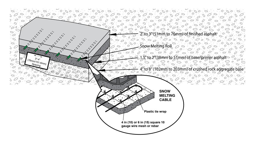
Note: Cables may be tied to reinforcement type mesh and then the mesh should be staked down to the base/primer layer.
