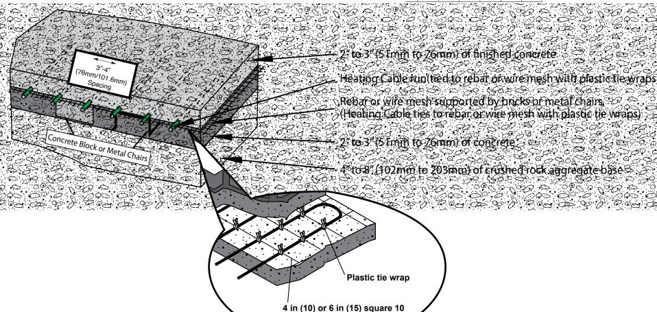
gauge wire mesh or rebar
