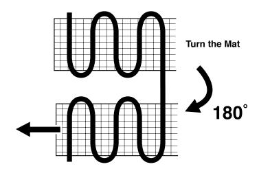
For other shapes, detach Cable from Mat to required length and lay only Cable.
