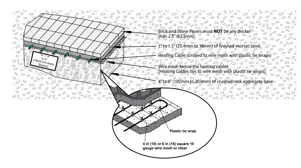
Note: Cables may be tied to reinforcement type mesh and then the mesh should be staked down to the base/crushed rock aggregate.
