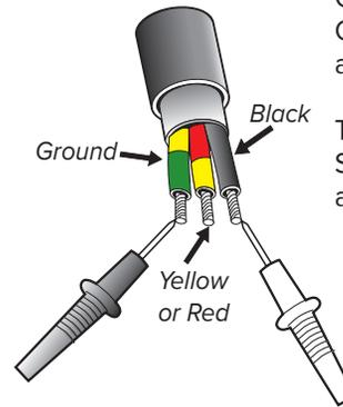
Connect the probes to both the Core wire and the Ground wire at the START of the lead.
