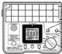
Connect the black test lead to the measurement terminal labeled EARTH.
