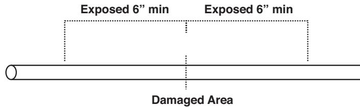
3. Cut the heating cable from each side of the damaged section such that there is a 4-3/4" gap between the heating cables.
