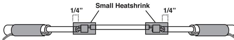
10. Slide the large heatshrinks over the small heatshrinks such that they extend a minimum of 1/4" beyond the edges and carefully heat to shrink them into place (the glue from the heatshrink will start to seep out of the end when shrinking is near completion) and then allow to cool to room temperature
