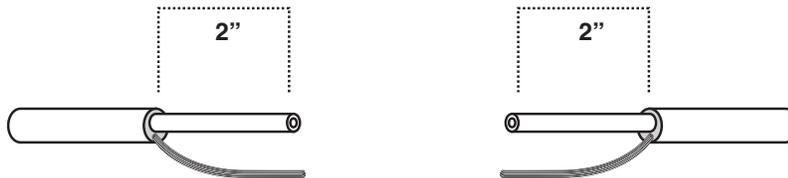
6. Fold the pigtails back and slide one small and one large heatshrink over each side of the heating cable.
