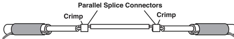
9. Slide the small heatshrinks over the connectors such that they extend a minimum of 1/4" beyond the edges and carefully heat to shrink them into place (the glue from the heatshrink will start to seep out of the end when shrinking is near completion) and then allow to cool to room temperature.
