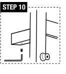
**STEP 10:** As shown in the picture, install the set screws (c) into the hole of all the tubes (a) using the allen wrench; fix the tube (a) onto the mounting bracket (g).
