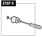
STEP 9: Insert long screw (i) through mounting bracket (g), then screw into plastic drywall anchor (f).
