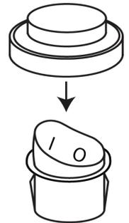
Re-attach wires to tabs. Push cover down onto the switch so it covers and fits over edge of the trim ring.
