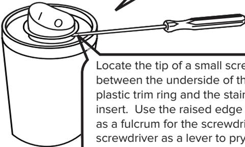
Locate the tip of a small screwdriver between the underside of the black, plastic trim ring and the stainless tube insert. Use the raised edge of the tube as a fulcrum for the screwdriver. Use the screwdriver as a lever to pry the switch out of the tube insert.
