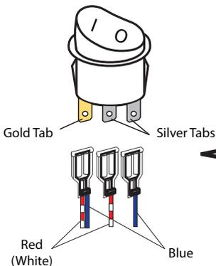
The push-on terminal with the two wires attached to it is attached to the gold tab of the switch. The red(white) push-on terminal gets attached to one silver tab and the blue terminal attaches to the last silver tab. There is no polarity with these 2 connections.
