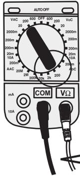
Check the Ohm meter to make sure that it contains fresh batteries and is set to a scale of 0 - 200 prior to taking any reading.
