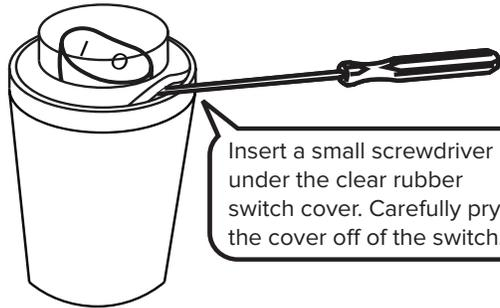
Insert a small screwdriver under the clear rubber switch cover. Carefully pry the cover off of the switch.
