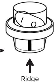
Note ridge in switch and match to groove in tube insert. Push switch down into tube insert until seated.
