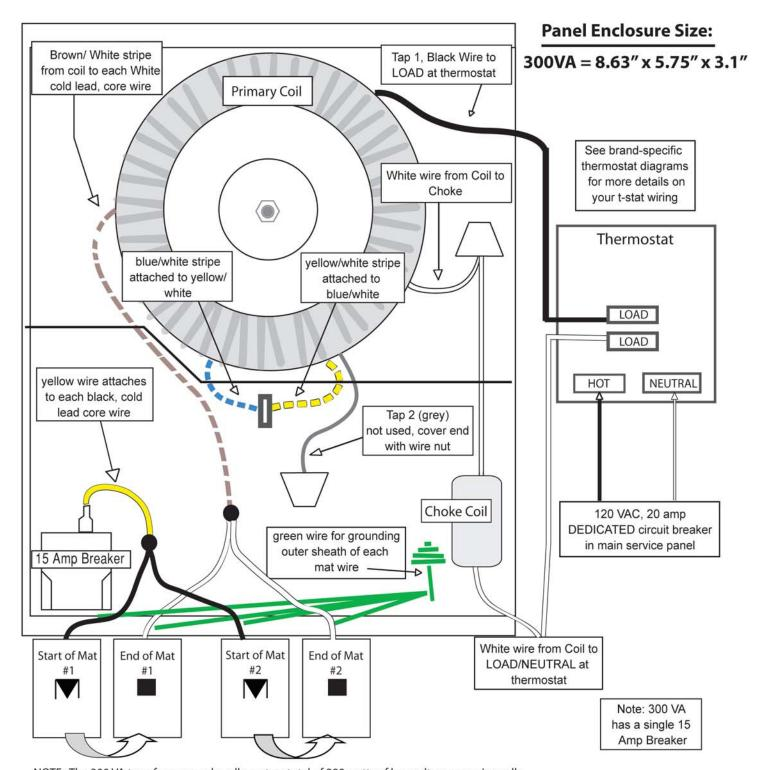
NOTE: The 300 VA transformer can handle up to a total of 300 watts of low voltage warming rolls. If the total watts requirements of all the rolls exceeds 300 watts, a larger capacity transformer will be needed.
