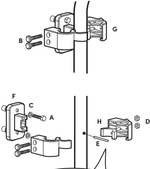
Insert the Pin through the hole on the tube before assembling the sleeve
