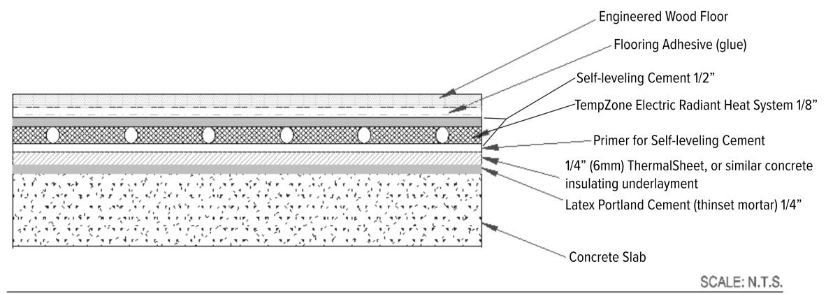
Application: Glued Engineered Wood over Insulated Concrete.
