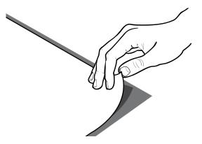
D. Move the heater from the top of the countertop and begin attaching it to the underside of the stone counter while keeping the white release liner on the heater. This is generally accomplished by sitting on the floor facing outward with your back to the cabinet.
