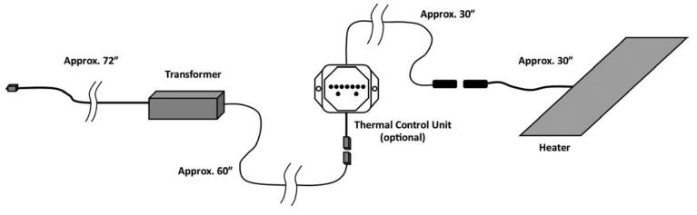
It is common to put the Thermal Control Unit within a cabinet or out of normal visibility but still accessible for periodic use. The Thermal Control Unit can be mounted onto the inside wall of a cabinet with the screws provided. The transformer typically lies in a cupboard or in the bottom of the cabinet. The transformer may feel warm to the touch (or a bit hot in some cases) this is normal.
