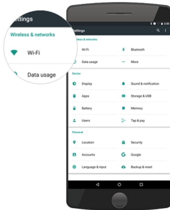
**Step 3:** Locate and connect to the Wemo with the same Wemo ID found at the back of the Wemo unit you are trying to install. The Wemo ID is the word **WeMo** followed by the Wemo model, then **three** alphanumeric characters. For example, **WeMo.Insight.xxx**. Also, the Wemo device is not secured thus, it will not ask for a password when you try to connect to it upon installation.
