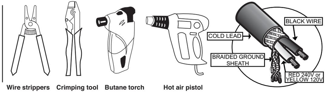
**Step 1** - Using a blade, strip 1" of the outer insulation from both cables.
