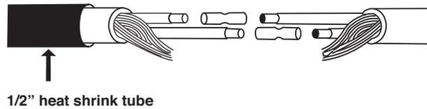
**Step 7** - Compress the crimp-on connector on each side using crimp tool. Using a butane torch, carefully heat crimp connectors to seal crimp and melt solder. Place the grounds into the uninsulated connector and crimp them together.
