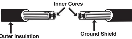
**Step 3** - Separate the braided sheath wire from the inner layers of insulation.
